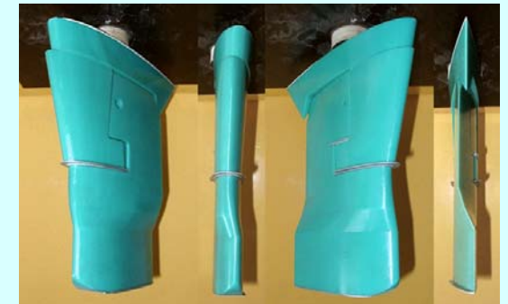
Semi-spade rudder modified to reduce cavitation
