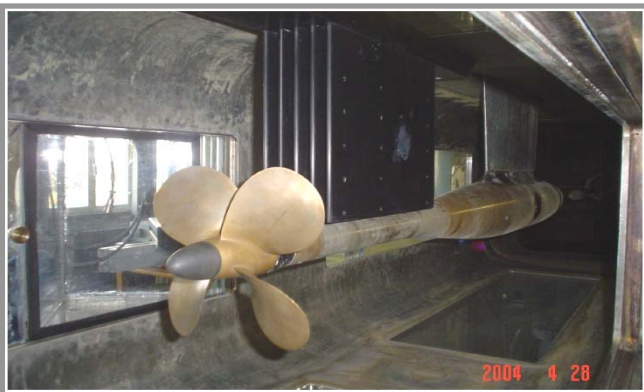
Propeller behind wake generator Italian Navy Cavitation Tunnel (CEIMM)
