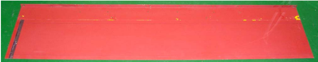
General SPC Paint (roughness~38 \mu m)
