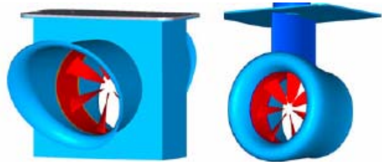
Rim-Driven Hubless Composite Inline Props (Büchler and Erdman, 2006)
