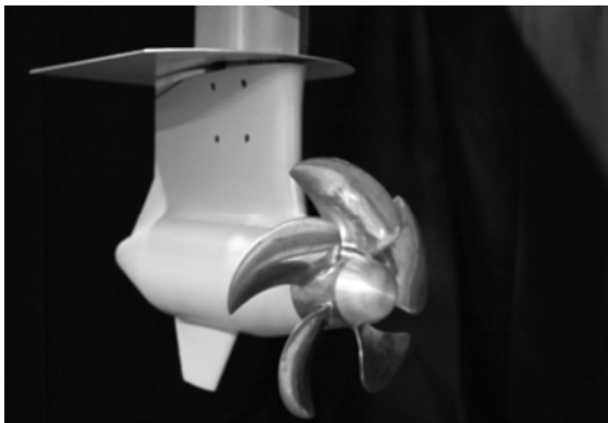
Figure 5.5: Typical pod unit open water test setup
