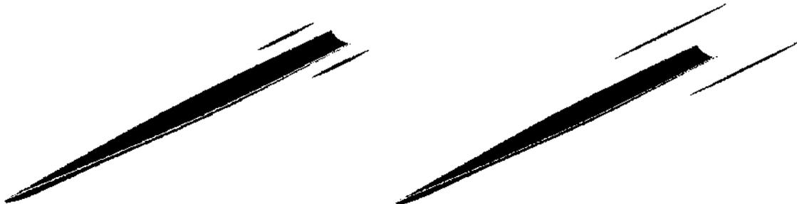
Fig. 1 Trimaran model (1%  $\nabla$  outrigger and 3%  $\nabla$  outrigger)
