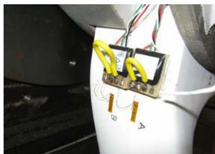
Fig. 3 Position of strain gauges.
