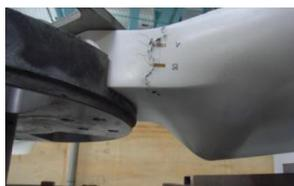
Fig. 1 Fatigue crack initiation.
