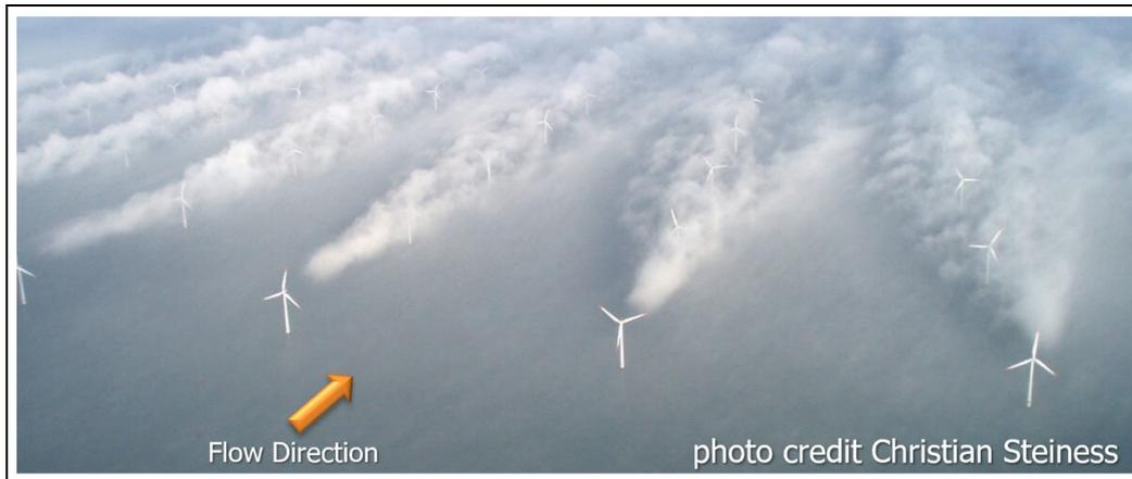
**Figure 1.** Aerial view (photograph) of wake clouds at Horns Rev I offshore wind farm 12 February 2008 at around 10:10 UTC, as seen from the southeast.
