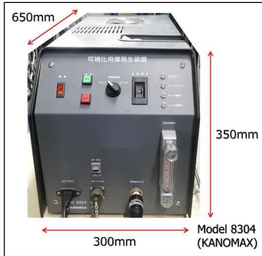
Figure 9. Smoke generator used in this study.
