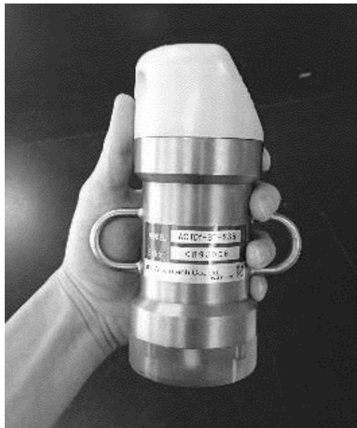
Figure 2.1 Photo image of new CTD sensor “S-CTD”. This CTD instrument allows Bluetooth communication with Android devices aiming at automatic data transfer.
