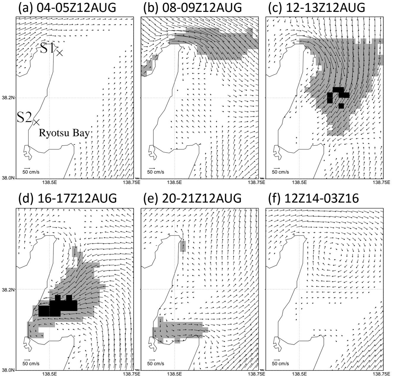
Sequence of surface velocity change associated with Typhoon 1004 (DIANMU). The five diagrams (a-e) are given by one-hour averages but the last one (f) is 39 hour (~ 2 inertial cycles) mean. Weak motions smaller than 10cm/s are omitted. Gray and black grids show normalized speeds larger than 4 and 8, respectively.
