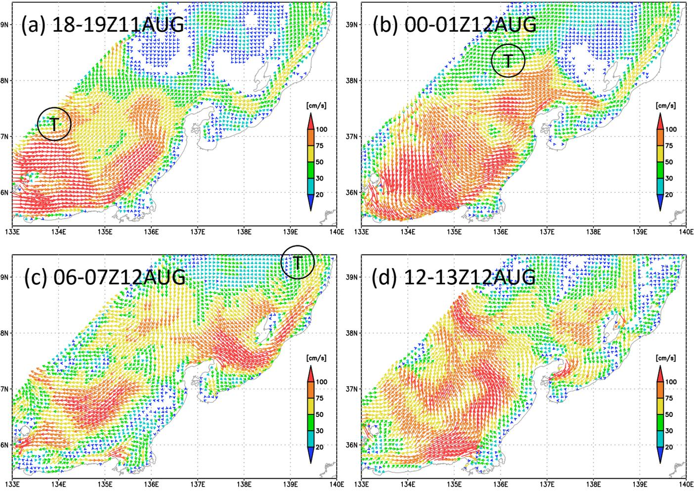
Simulated velocity distribution by the DR\_C model at 10m depth under the passage of Typhoon 1004 (DIANMU). The vectors are plotted at 5 grid interval (~7.4km). The magnitude is given by the color scale shown in each diagram. Any motion weaker than 10cm/s is omitted.
