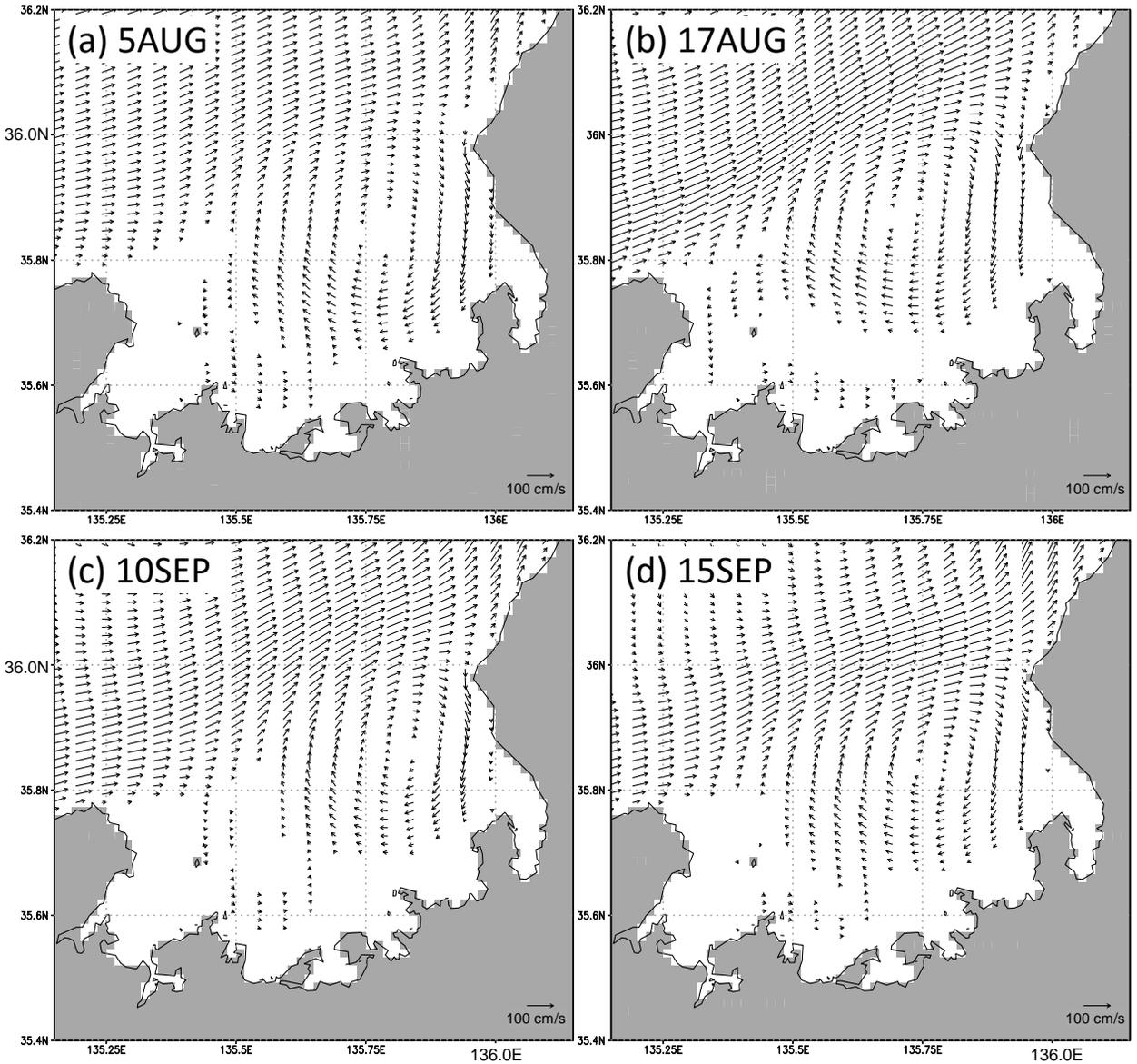
Horizontal velocity field at each maximum growth of the warm eddy at 10m depth in Wakasa Bay. These velocity components are based on 21-hour (~inertial period) averages from 1:00Z to 22:00Z at (a) 8/5, (b) 8/17, (c) 9/10, and (d) 9/15 of 2010. The speeds smaller than 10cm/s are eliminated.
