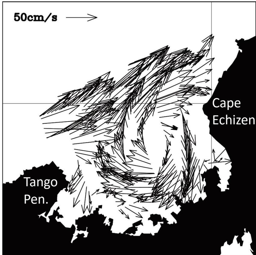
Horizontal velocity measured by ADCP of R/V Fukui-maru on September 16, 2010. The vector scale is shown at the northwestern part.
