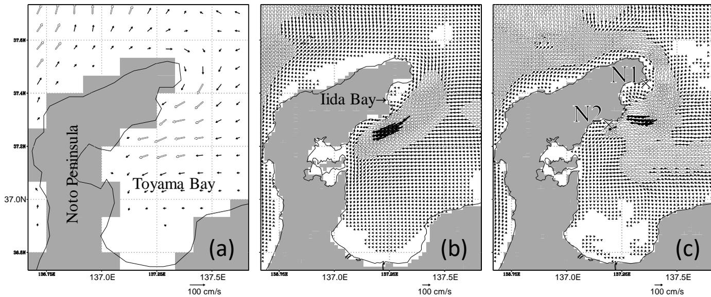
Horizontal velocity field at 10 m depth at the time of a kyucho arrival to Stn.N2 (06-07Z of 7/12, 2010) in Toyama Bay modeled by (a) DR\_M, (b) DR\_I, and (c) DR\_C. The open and thick vectors show the speed larger than 50 and 100cm/s, respectively. Weak motions smaller than 10cm/s are omitted.
