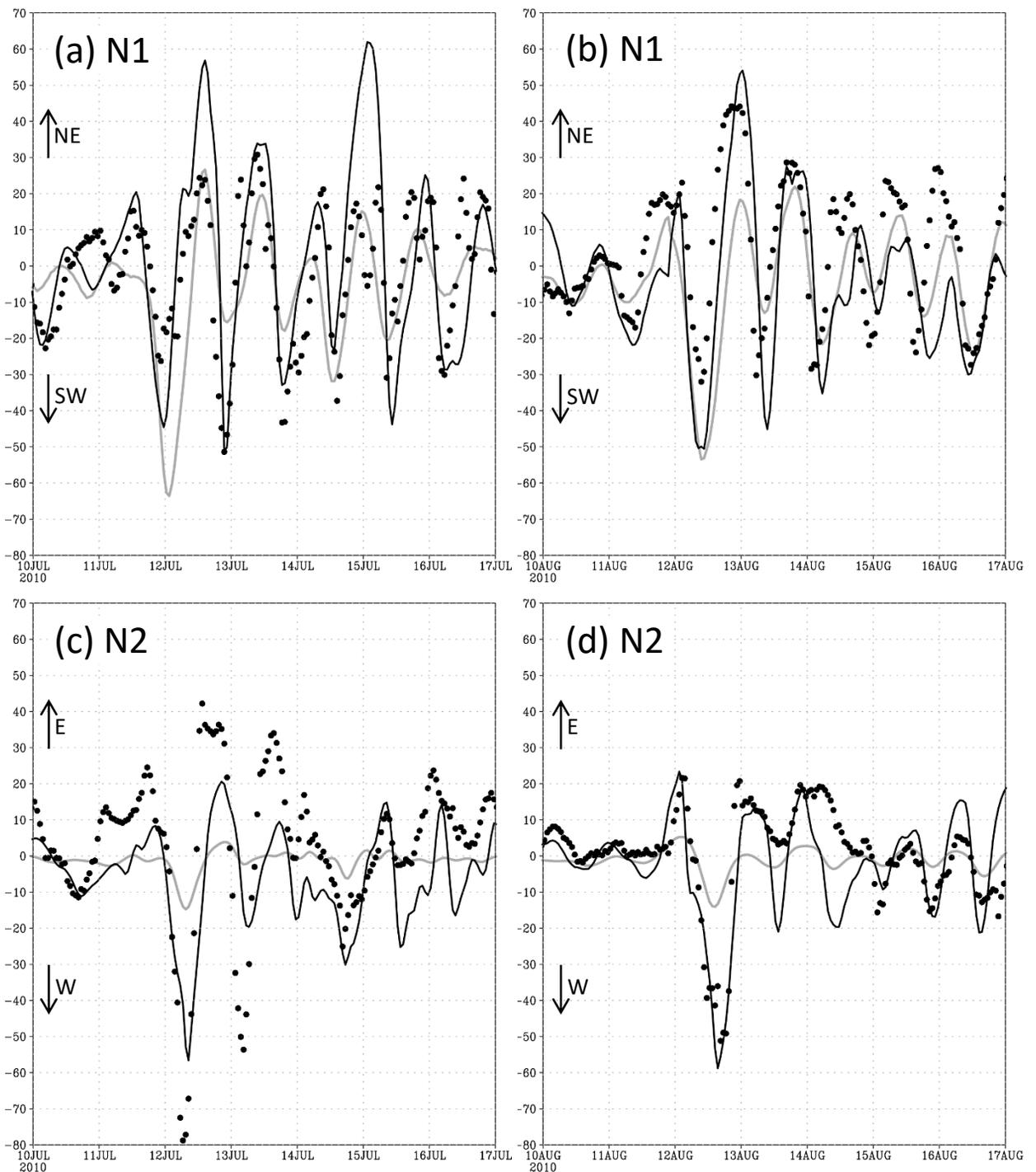
Time series of alongshore velocity component in cm/s for one week from 00Z of (a,c) July 10 or (b,d) August 10 at 10m depth at (a,b) N1 of  $37^{\circ}26'N$ ,  $137^{\circ}22'E$  and (c,d) N2 of  $37^{\circ}17'N$ ,  $137^{\circ}11'E$ , whose locations are indicated in the previous figure. The gray and black curves show the parent and child model (DR\_M and DR\_C) results, respectively. The dots are given by in-situ measurement.
