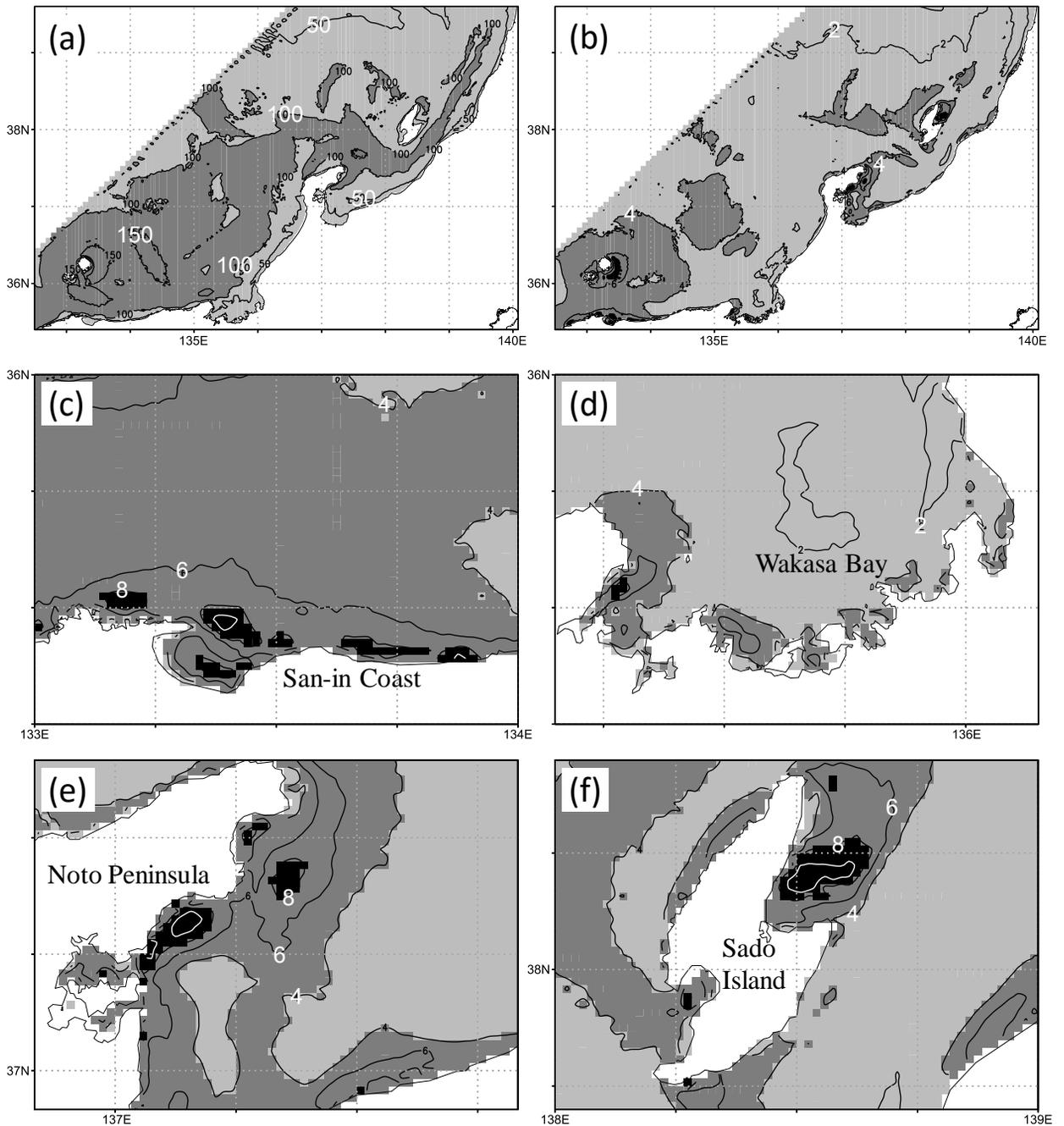
(a) Maximum water speed at 10m depth during the three days from 00Z 8/11, 2010 with a contour interval of 50cm/s. (b-f) Same as (a) but divided by the scalar average over three month from July to September, 2010. The contour interval is 2.
