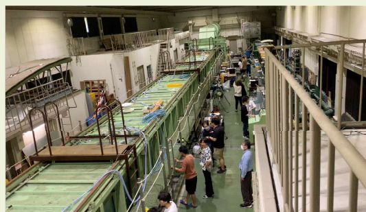
成層発生装置付きの台風シミュレータ(風洞波浪実験水槽) Typhoon simulator (wind-wave flume) with a thermal stratification generator
