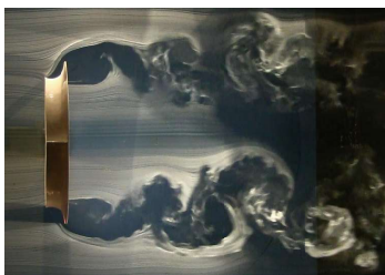
温度成層風洞で行ったスモークワイヤー法によるレンズ風車の集風体周りの流れの可視化実験 Visualization of flows around a shrouded wind turbine in a thermally stratified wind tunnel using the smoke wire method
