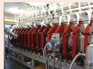
プラズマ乱流実験装置 (PANTA) Plasma Assembly for Nonlinear Turbulence Analysis
