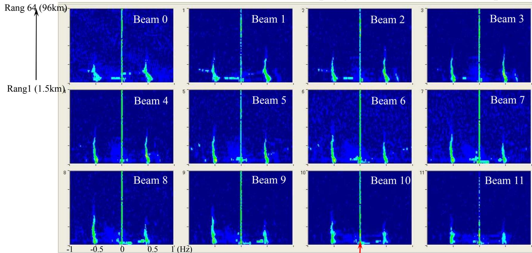
Internal noise emitting from the inside of the radar
