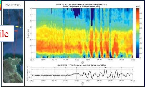
Fig. 1. Left panel: Used beam (15°) for the plot on the right panel. The direction of the approaching tsunami is marked yellow, the size of the measured pixel is marked red.
