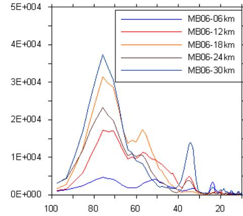
The radial velocities offshore have much power in the 30-40min band
