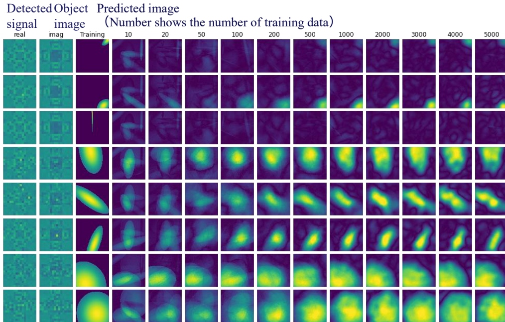
Fig. 2. (a) Received microwave signals, (b) object surface images and (c) corresponding reconstructed surface images by models with different numbers of training data. The input channels take real part and imaginary part of complex amplitudes. The numbers above images show the numbers of training data.
