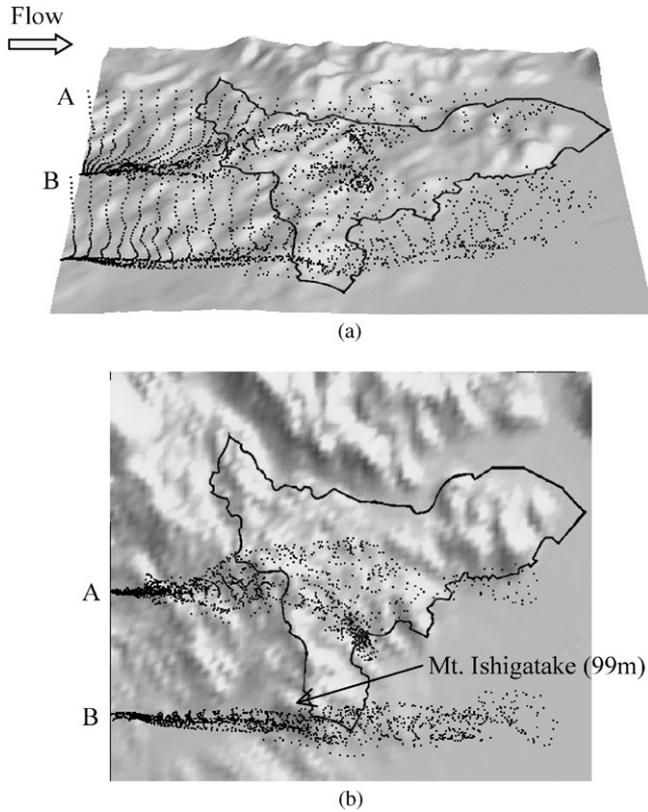
Fig. 8. Particle movement released at two upstream positions of the new campus area: (a) side view; (b) top view. A non-dimensional time interval is  $\Delta t = 0.4$ , and this figure was obtained after 20 intervals.
