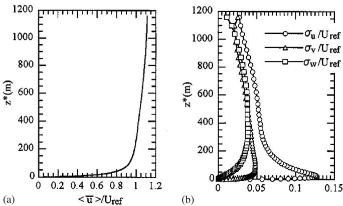
Fig. 7. Turbulence statistics in the upstream driver unit: (a) mean-velocity profile; (b) turbulence intensities in the  $\underline{x}$ -,  $\underline{y}$ -, and  $\underline{z}$ -directions. All the quantities are time- and spanwise-averaged at  $x = 76 h$  from 200 non-dimensional time units.
