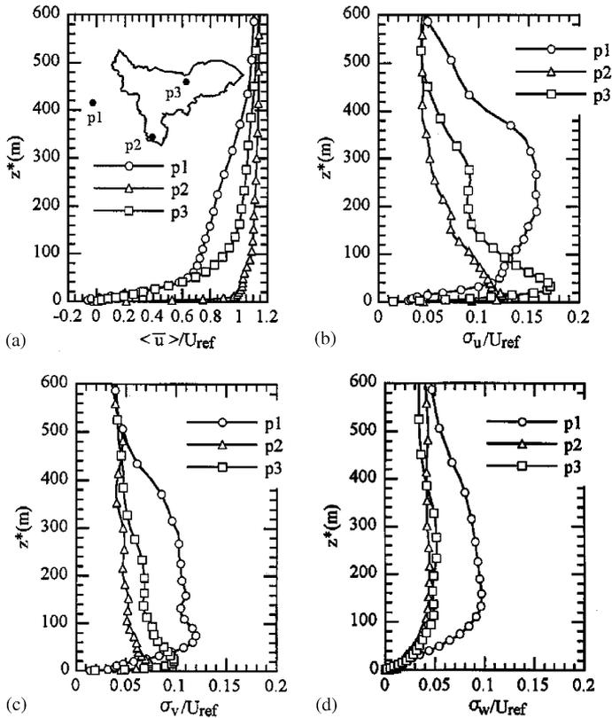
Fig. 9. Turbulence statistics at three different locations, i.e., p1, p2, and p3: (a) mean-velocity profile; (b–d) turbulence intensities in the  $x$ -,  $y$ -, and  $z$ -directions. All the quantities are estimated from 100 non-dimensional time units.
